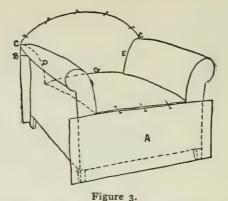
This diagram should be studied in conjunction with the text as it shows how and where to pin pieces together.
